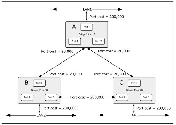
Figure 4-6-2: Before Applying the STA Rules
