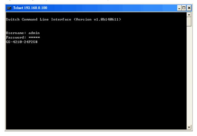
Figure 5-4: Telnet Login Screen
