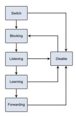
Figure 4-6-1: STP Port State Transitions
