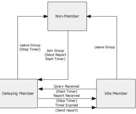
Figure 4-7-6: IGMP State Transitions
