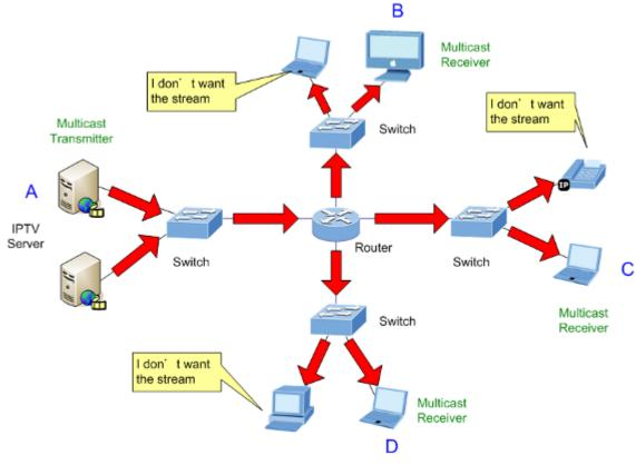
Figure 4-7-4: Multicast Flooding
