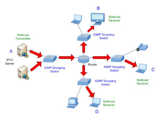
Figure 4-7-5: IGMP Snooping Multicast Stream Control
