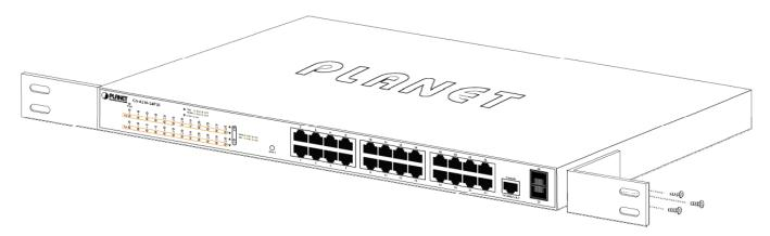
Figure 2-1-10: Attach Brackets to the Managed Switch
