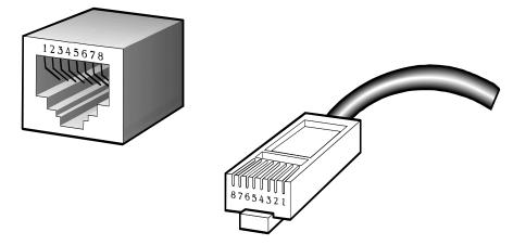
The standard RJ45 receptacle/connector
