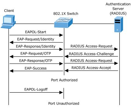
Figure 4-9-6: EAP Message Exchange
