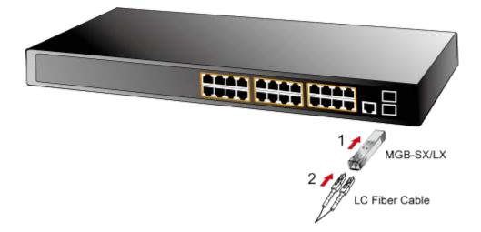
Figure 2-1-12: Plug In the SFP Transceiver
