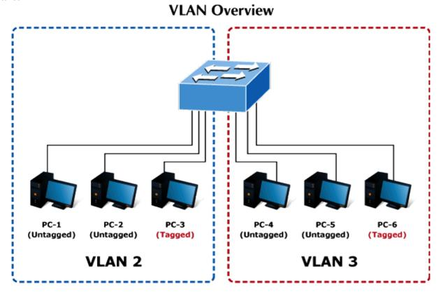
Figure 4-5-20: Two Separate VLAN Diagrams
