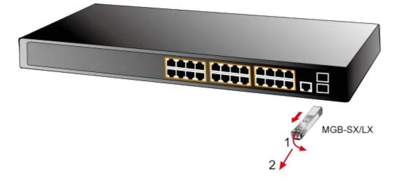
Figure 2-1-13: How to Pull Out the SFP Transceiver
