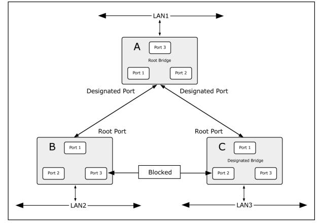
Figure 4-6-3: After Applying the STA Rules
